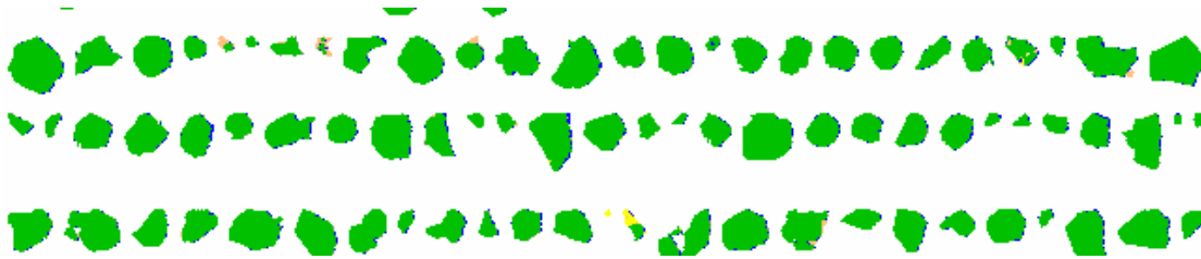
Qemscan data showing very low impurity levels.
